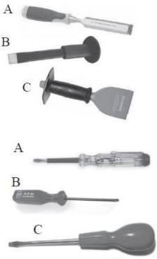
Here are three types of chisel. Chisel A is used for cutting soft materials, such as wood, and chisel B is used for cutting metal. Chisel C is for cutting away old plaster and brickwork.
